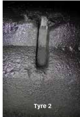
Tyre wear after 16 months' usage.
