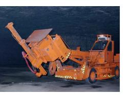
The Fletcher Series 3100 Roof Bolter is designed for bolting in high roof conditions up to 10.6 meters. Tramming is done from the enclosed cab. Drilling, resin insertion, and
