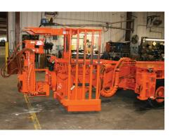
Fletcher Model HDR is a versatile roof drill designed for general purpose bolting in up to 4.5 m high roof conditions. The model HDR features an operator platform, therefore rib
