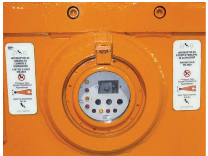
Diagnostic indicator lights in main controller
