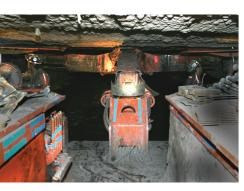
With Fletcher model DDR Walk-Thru, you get dual head, angle or vertical drilling in lower seams than ever. Model DDR offers a maximum straight line boom swing of 5.4 m to accommodate a 4 bolt pattern on 1.2 m centers. Masts tilt 45 degrees for truss installations; 90 degrees for tramming.
