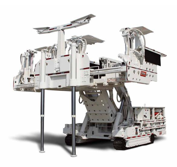
The Fletcher CHDDR-4 is a four mast feed roof drill. The bolter is run by two operators, each working two separate drill masts. With operator slide out platforms, operators can use detented controls to bolt the inside, outside, and toward the rib. Because the masts operate independently from each other, operators can simultaneously perform separate tasks, maximizing production time.
