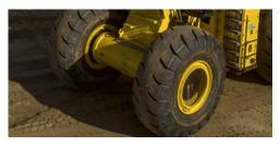
Komatsu pressurized axle housings enhance reliability by maintaining an air-cooled, dust-free environment for the traction motors and disc service brakes.
