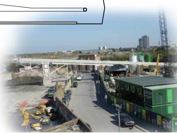
HAC system technology has solved many high capacity, steep angle conveying problems, up to and including vertical lifts. The HAC system employs standard conveyor idlers and rollers and a proven sandwich-belt principle that overcomes the limitations typically encountered with many traditional methods of conveying.
