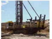
The P&H 285XPC provides up to 53,524 kg (118,000 lbs) of bit loading specifically designed for 270 and 311 mm diameter hole applications. This drill is well suited for the majority of copper and iron applications.
