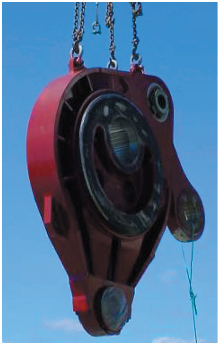
Straddle-supported, eccentric design walk leg and knee mechanism for P&H 9000C-series draglines.
