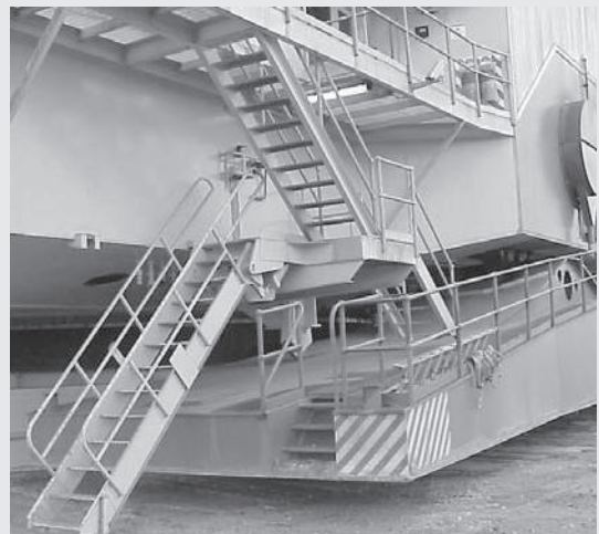
The air-operated boarding stairway helps facilitate easier dragline boarding and dismounting, especially for maintenance personnel carrying tools, supplies and parts.
