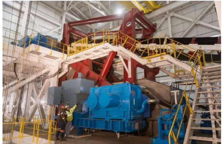
Once the system was in regular operation excessive startup torque was detected during the continued monitoring. The Smart team then used those baseline readings to quickly target the problem area.
